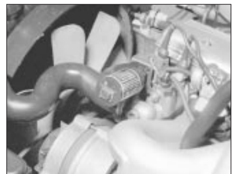
34.2b An aftermarket service light resetting tool such as this one can be plugged into the service connector and used to reset the service lights
