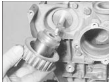
14.8 Removing the timing belt tensioner (M40 engine)
