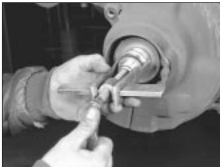
8.8b If the inner race of the bearing sticks to the stub axle, use a puller to get it off
