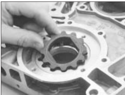
14.22a Removing the inner rotor . . .
