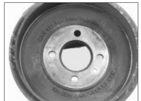
6.3 The maximum allowable inside diameter of the drum is cast into the drum
