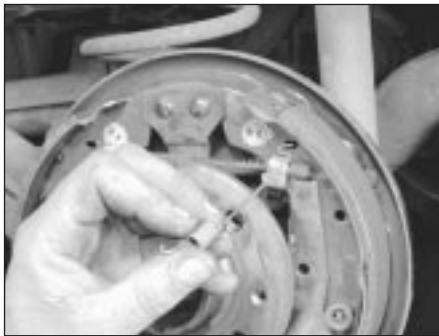
6.5b . . . then unhook it from the rear shoe and remove it
