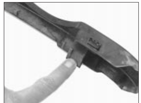
9.10 Detach the centre grille valance by reaching under each headlight and pressing on the release lever
