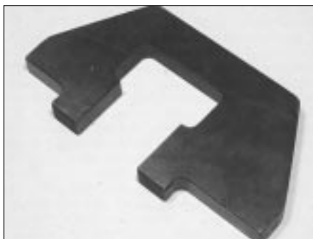
10.11a The BMW tool for holding the camshaft in the TDC position on M40 engines
