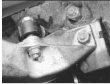
17.6 Engine mounting and damper on the M40 engine
