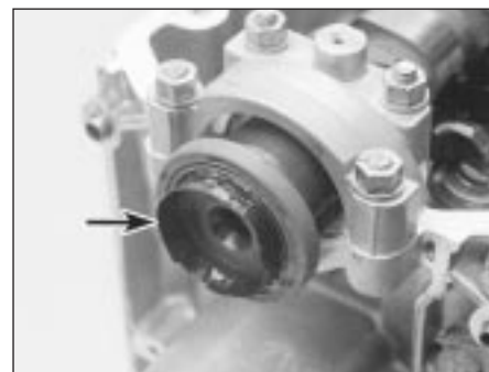
11.14 Fitting a new camshaft oil seal on the M40 engine (note the adhesive tape around the end of the camshaft to protect the seal)
