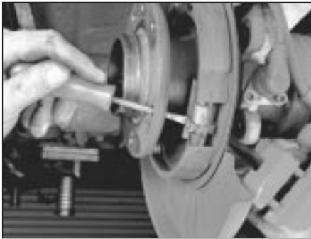
5.6d If a rear disc still sticks to the hub, insert a thin, flat-bladed screwdriver through the hub flange, rotate the starwheel on the handbrake adjusting screw, and contract the handbrake shoes (disc removed for clarity)
