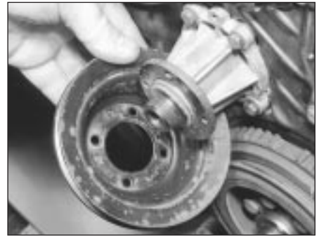
5.29 Removing the water pump pulley (M40 engine)
