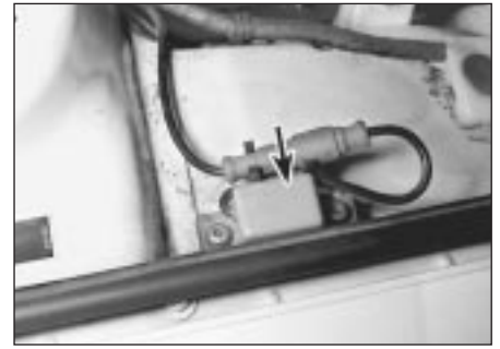
18.3 The SRS system crash sensors (arrowed) are located in the engine compartment - check the wiring regularly for damage
