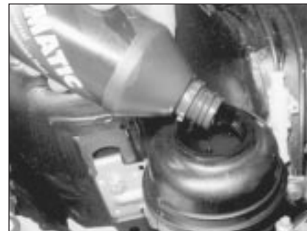
7.6 Adding fluid to the power steering reservoir
