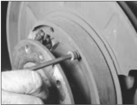
12.7c Remove the shoe hold-down springs
