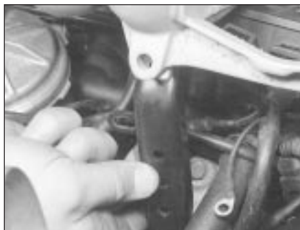
5.12 Removing the support bracket from the bottom of the intake manifold (M40 engine)
