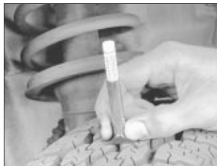
5.2 Use a tyre tread depth indicator to monitor tyre wear - they are available at car accessory shops and service stations, and cost very little
