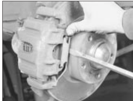
3.5h Prise off the anti-rattle spring (5-Series)
