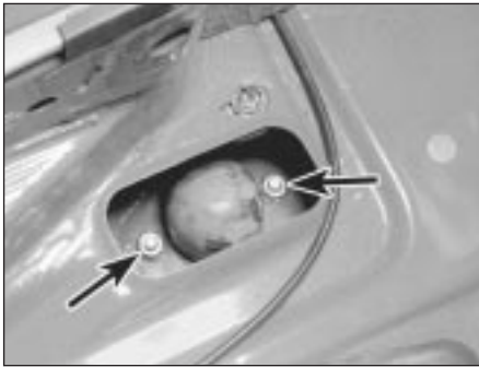
9.4 Shock absorber upper mounting nuts (arrowed) - late-model convertible shown. On other early models, upper nuts are accessible from the luggage compartment; on later models, they're behind the back of the rear seat, up under the parcel shelf
