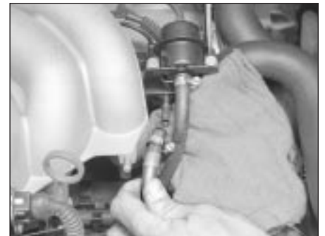
2.4 Be sure to place a rag under and around any fuel line when disconnecting
