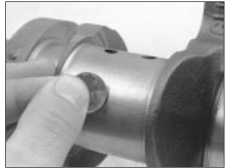
19.4 Rubbing a penny lengthways on each journal will reveal its condition - if copper rubs off and is embedded in the crankshaft, the journals should be reground
