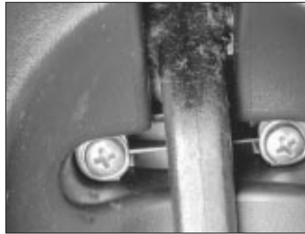
19.4 The lower screws are located under the tilt lever (where fitted)
