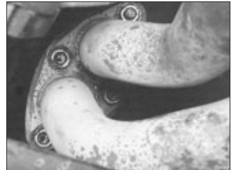
6.5b Exhaust manifold-to-downpipe flange (M40 engine)
