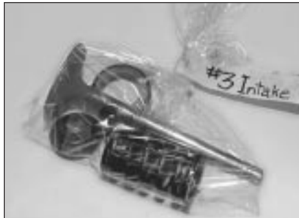
8.21 A small plastic bag, with an appropriate label, can be used to store the valve components so they can be kept together and refitted in the original position
