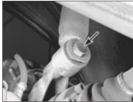
11.2 Remove the shock absorber lower mounting bolt (arrowed)
