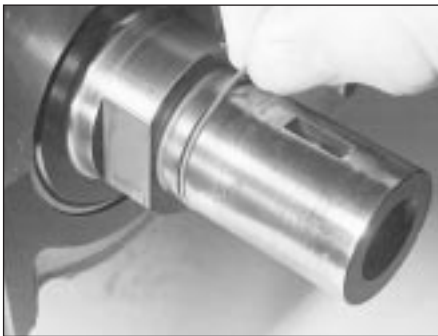
14.14b Extract the rubber O-ring from the groove in the nose of the crankshaft (M40 engine)
