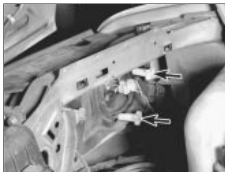
13.1 The headlight adjustment screws (arrowed) are accessible from the back of the headlight on 3-Series models
