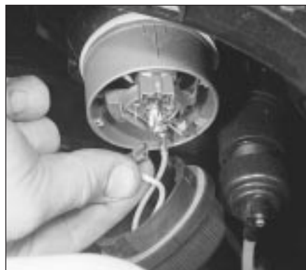
12.10 Disconnecting the wire from the rear of the headlight bulb
