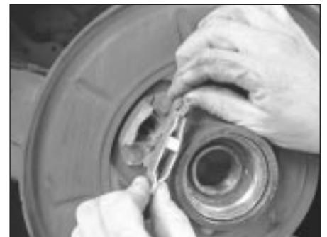
10.4a To detach the handbrake cable from the handbrake actuator on models with rear disc brakes, pull on the outer cam and disconnect it from the inner cam . . .
