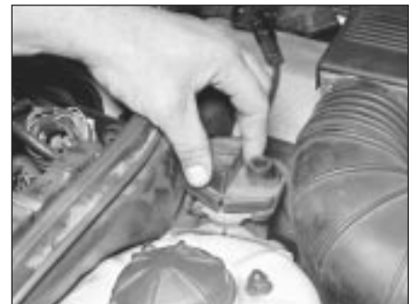
9.4b Some Motronic systems use a different type of coil. First, remove the coil cover and . . .
