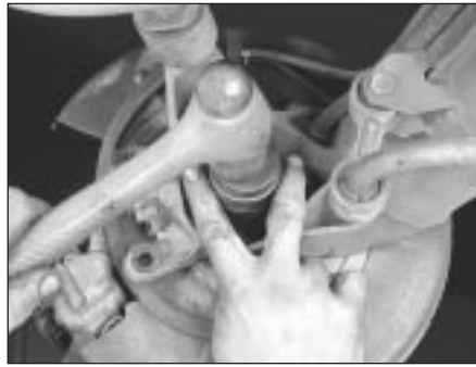
15.13b . . . then drive the bearing out of the housing with a large socket or a suitable piece of pipe
