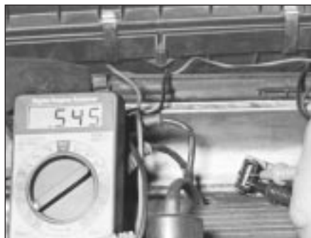
12.8 The resistance of the pulse sensor should be 500 to 600 ohms (later models)
