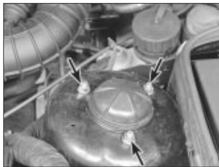
5.13 Support the weight of the strut and remove the three mounting nuts (arrowed) at the top of the strut (5-Series shown, 3-Series similar)
