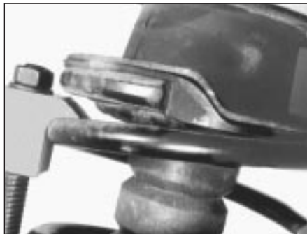
6.11 Make sure you align the end of the coil spring with the shoulder of the rubber ring, and with the spring retainer
