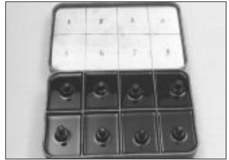
8.19 Compartmentalised box to hold the hydraulic tappets (M40 engine)
