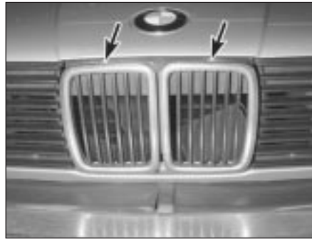
9.2a The centre grille is held in place by two screws (arrowed)
