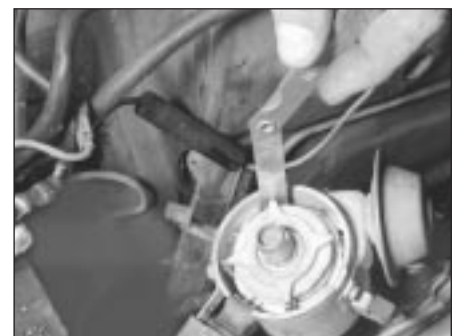
11.2 Use a brass feeler gauge to check the air gap (be sure the gauge rubs lightly against the trigger wheel as well as the locating pin for the correct adjustment)
