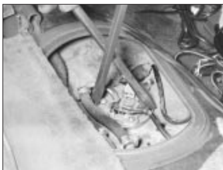
4.18a On models with locking lugs, use two screwdrivers to rotate the assembly out of the notches
