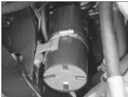
6.12 EVAP system charcoal canister viewed from under the vehicle (316i model)
