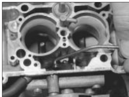
12.15a Choke linkage arm located in the automatic choke lever
