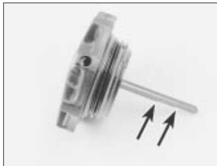
7.4 The power steering fluid level should be kept between the two arrows near the upper step on the dipstick
