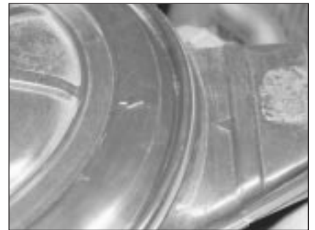
8.9 Align the air cleaner cover arrows when refitting
