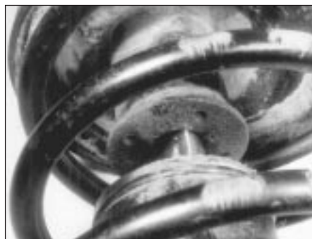
6.9 Loosen and remove the threaded collar, and pull the old strut cartridge from the strut housing - on all struts except gas-charged units, pour the old oil from the strut housing. (Spring should have been removed first)
