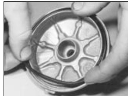
6.19 Renewing the rubber O-ring in the cover
