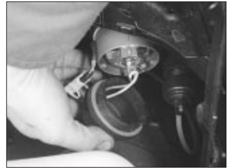
12.9 Twist and release the headlight inner cover
