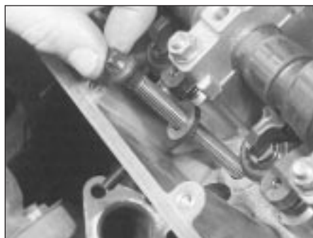
12.29 Inserting a cylinder head bolt (M40 engine)
