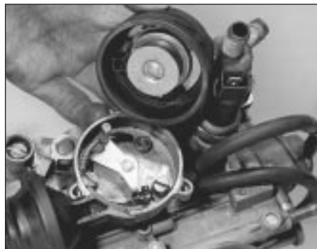
12.18 Remove the automatic choke cover, at the same time disengaging the bi-metal spring from the control lever
