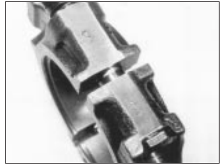
12.4 Mark the big-end bearing caps in order from the front of the engine to the rear (one mark for the front cap, two for the second one and so on)
