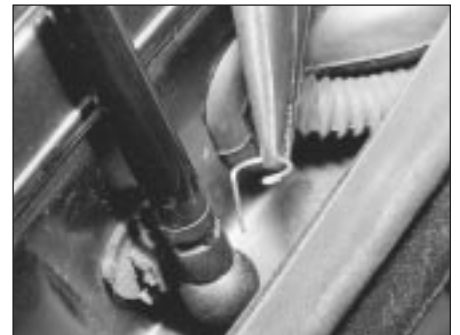
14.12c Removing the retaining pin to disconnect the bottom of the tailgate support strut (5-Series)
