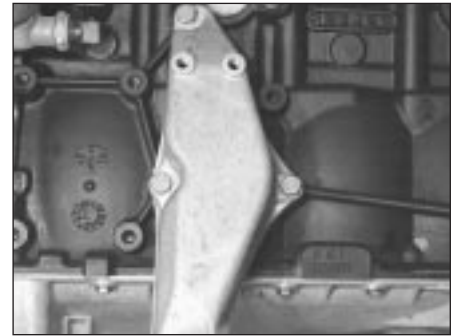
7.3 Engine left-hand mounting bracket - M40 engine
