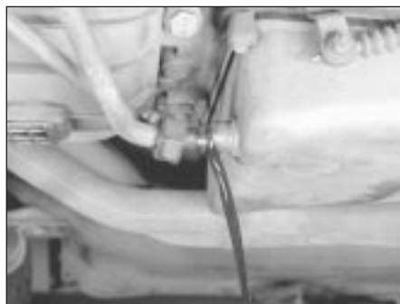
28.5b Detach the tube and let the fluid drain
