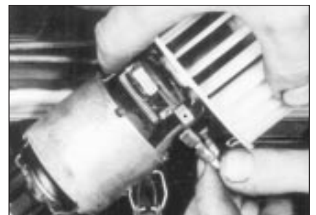
9.6 Lift out the assembly, and disconnect the electrical connection from the blower motor
