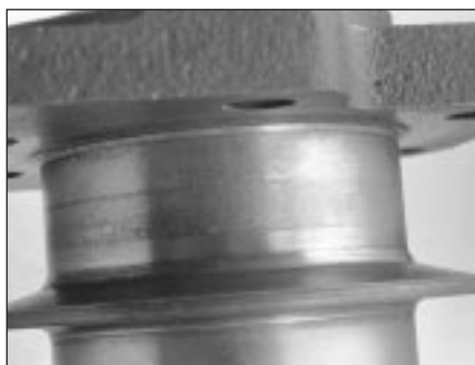
19.8 If the seals have worn grooves in the crankshaft journals, or if the seal contact surfaces are nicked or scratched, the new seals will leak
