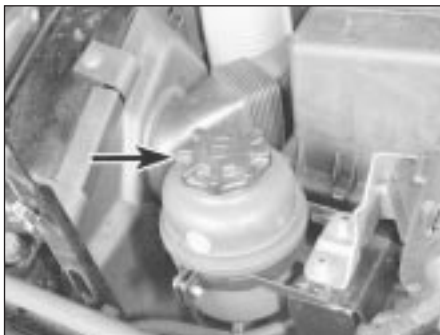
7.2 The power steering fluid reservoir (arrowed) is located on the left side of the engine compartment
