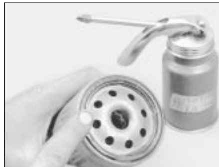
6.16 Lubricate the oil filter sealing ring with clean engine oil before refitting the filter on the engine
