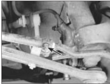
17.3 Loosen the clamp bolt (arrowed) that locks the track rod end to the inner track rod. Paint an alignment mark on the threads, to ensure the track rod end is refitted in the same position, and unscrew the track rod end from the inner track rod
