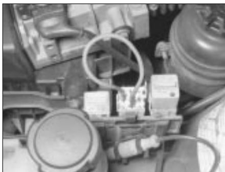
3.6b On Motronic systems, use a jumper wire to bridge the terminals on the connector that correspond to the fuel pump relay pins 30 and 87
