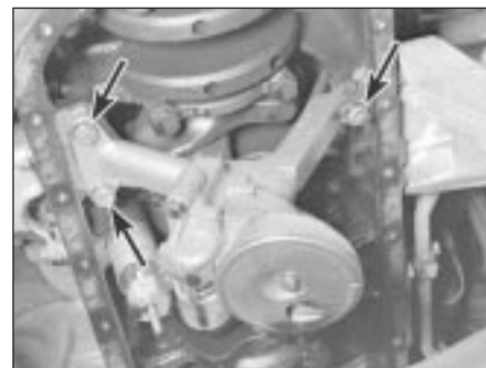
14.3a On M20 engines, the oil pump is bolted across the engine block from side to side, towards the front of the engine
