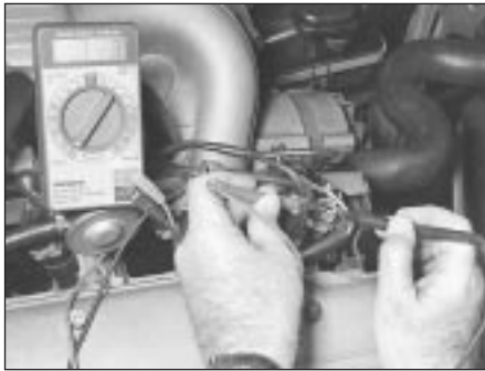
19.6 Check the resistance of the thermotime switch with the engine coolant temperature below 30° C. There should be continuity
