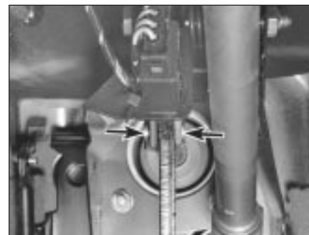
8.9 Disconnect the brake pedal return spring, then remove the clip and clevis pin (arrows) to disconnect the pushrod from the brake pedal (left-hand-drive models)
