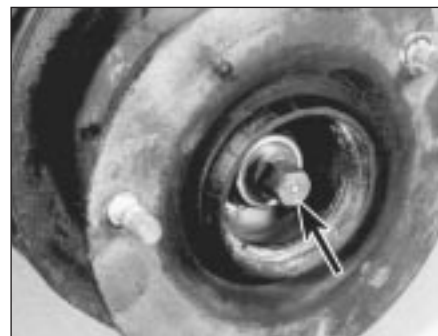
6.4 Prise the protective cap off the damper rod nut, and remove the large nut (arrowed) - to prevent the damper rod from turning, place an Allen key in the end of the shaft
