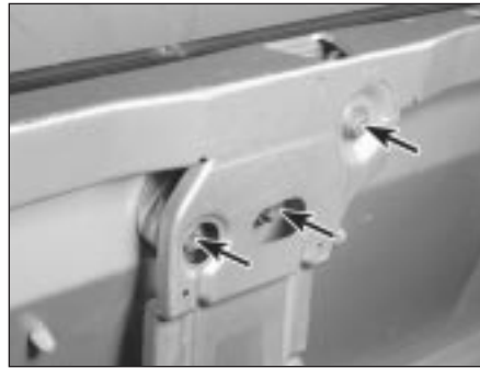
14.7a Loosen the lock bolts (arrowed) and move the lock to adjust the boot lid closing position
