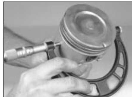
18.11 Measure the piston diameter at a 90-degree angle to the gudgeon pin, at the same height as the gudgeon pin
