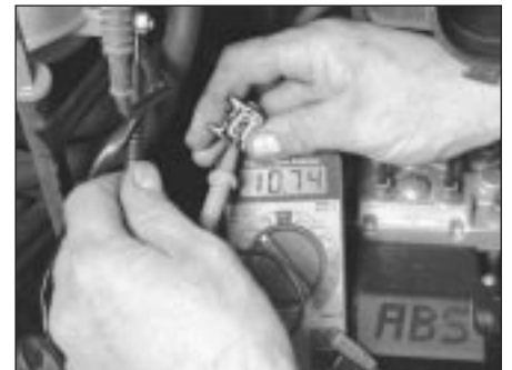
6.9 Check for battery voltage at the electrical connector to the purge valve
