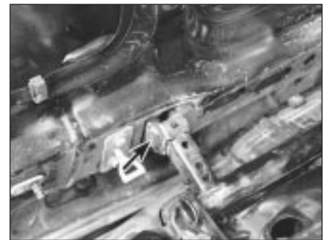
10.12 Unscrew the hinge through-bolts (arrowed)
