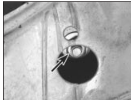
20.7 To unbolt the idler arm from the subframe crossmember, remove this nut (arrowed)
