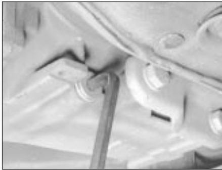
32.4 Remove the differential drain plug with an Allen key
