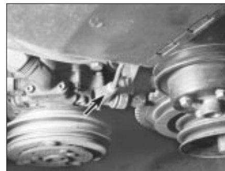
12.10 The pulse sensor itself (arrowed) is located on the timing belt cover, to one side of the pulley (later models)
