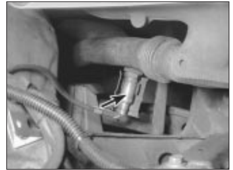
4.6 The oxygen sensor (arrowed) is usually located in the exhaust pipe, downstream from the exhaust manifold
