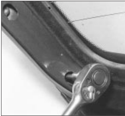
14.14 Unscrewing the hinge mounting bolts (5-Series)
