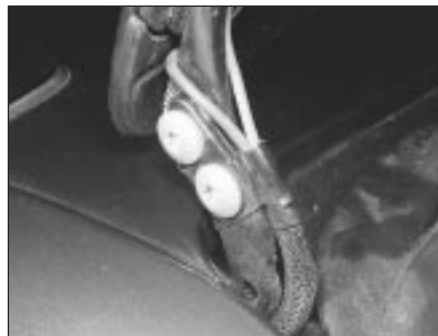
14.9 Tailgate window mounting screws (5-Series)
