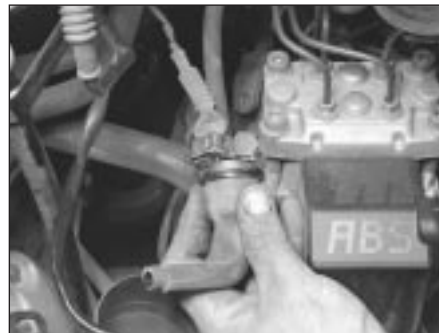
6.8 When the ignition is switched on, there should be a distinct "click" from the purge valve
