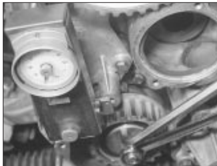
10.23a Using the special BMW tool to check the tension of the timing belt on the M40 engine
