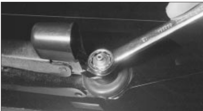
16.9 Removing the tailgate wiper arm nut (3-Series)
