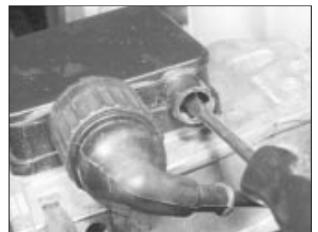
12.12b Adjusting the CO on the Motronic system
