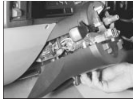
19.5a Pull the tilt lever down (where fitted), and lower the shroud from the steering column
