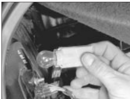
15.3a The tail light bulbs on later 5-Series models are in self-earthing holders which can be simply pulled out of the housing - the bulb is then removed from the holder
