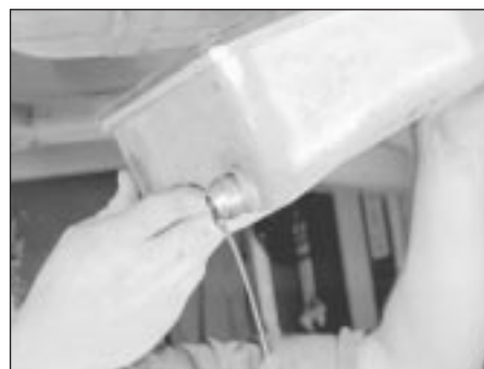
28.7 Lower the sump from the transmission
