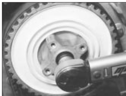
10.27 Tightening the camshaft sprocket retaining bolt on the M40 engine
