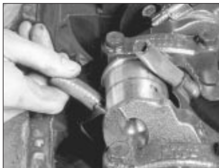
12.6 To prevent damage to the crankshaft journals and cylinder walls, slip sections of rubber or plastic hose over the rod bolts before removing the pistons
