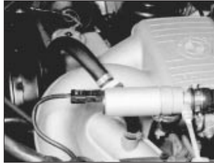
21.19 Location of the adjustment screw on the metal-type idle air stabiliser valve (L-Jetronic system)
