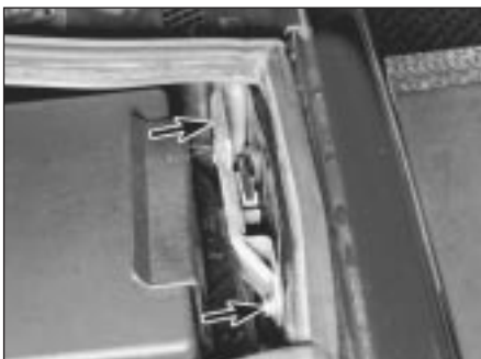
10.17 Loosen the bolts (arrowed) and raise or lower the catch to adjust the bonnet height
