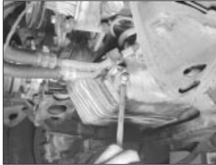
13.4 If applicable, remove the nut securing the power steering lines to the sump, and move the lines to one side to allow you to get at the sump bolts
