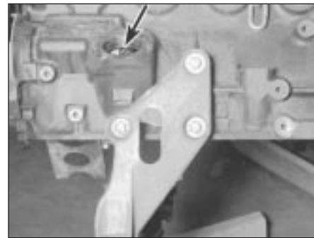
14.4 If necessary on the M20 engine, remove the plug and oil pump driveshaft from the engine. Inspect the driveshaft gear, as well as this intermediate shaft gear in the engine block (arrowed)
