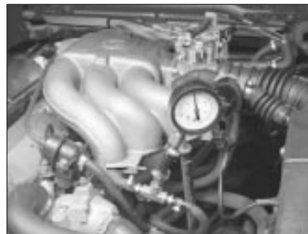
3.11 . . . and connect the gauge between the fuel feed line and the fuel rail using a tee-piece fitting
