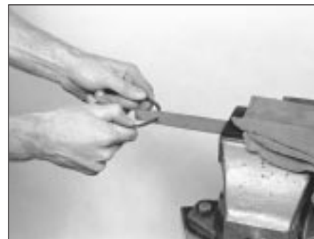
22.5 If the end gap is too small, clamp a file in a vice, and file the ring ends (from the outside in only) to enlarge the gap slightly
