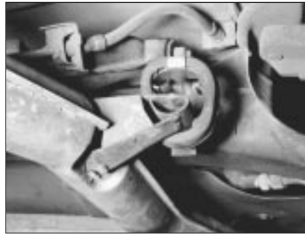
22.1 A typical exhaust system rubber mounting
