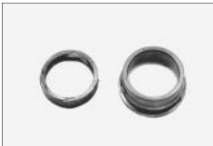
15.14b You can fabricate your own spacer tool from a piece of 13 mm long, 38 mm inside diameter pipe (left); you'll also need to use the old inner race (right)
