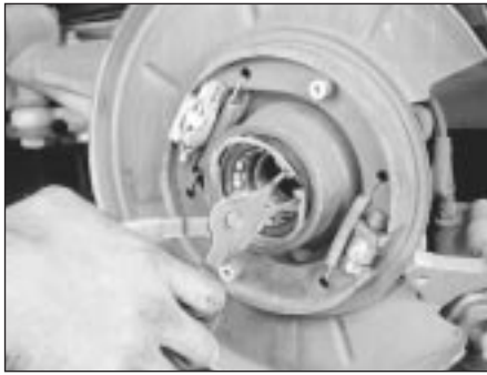
15.13a Remove the large circlip that retains the bearing in the housing . . .
